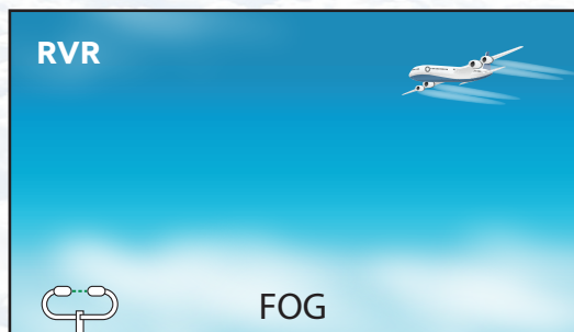
Runway Visual Range (RVR) is currently measured in-situ on the runway
